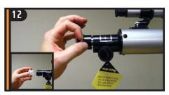
Loosen the set screw on the focuser and remove the plastic cap.
