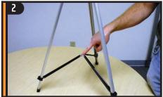
To set up the tripod, spread the legs outward until they are fully extended. Extend the center portion of each of the three tripod legs down 6-0"
