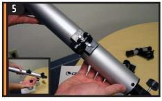
Remove the threaded bolt from the underside of the telescope tube.
