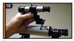
Orient finderscope so that it is facing toward the front of the tube. Place finderscope over screws as shown above.
