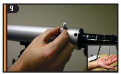
Remove knurled finderscope nuts from the optical tube.
