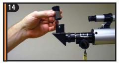
Place the 20mm eyepiece into the barrel of the diagonal as shown above. Tighten the set screw to secure in place.
