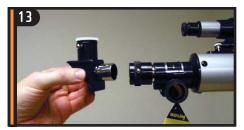
Insert the diagonal into the focuser and tighten the set screw to secure in place. Remove the plastic cap on the diagonal.
