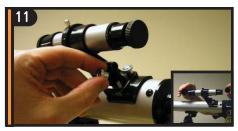
Replace knurled nuts to secure in place and remove lens covers.
