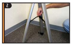
To set up the tripod, spread the legs outward until they are fully extended and push down center leg brace. Extend the center portion of each of the three tripod legs down 6-8".
