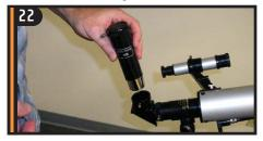
For additional magnification, you can use the included 3x barlow. Place the barlow in the focuser in place of the eyepiece - remove the cap from the barlow.
