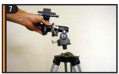
Locate the equatorial mount and place the base of the mount through the hole in the center of the tripod mounting platform.
