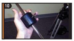
Locate the counterweight bar and counterweight. Slide the counterweight half way down the counterweight bar and tighten the wingnut to secure in place.
