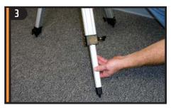
Use the three tightening screws located at the bottom of each leg to secure the extended legs in place.
