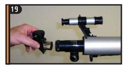
Loosen the set screw on the focuser so that it does not obstruct the inner diameter of the focuser. Insert the chrome barrel star diagonal into the focuser and tighten the set screw.
