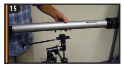
Place the tube on the mount by lining up the screws with the mounting holes on the mount.
