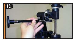
Slide the chrome end of the slow motion control cable onto equatorial mount gear shaft and tighten set screw to secure in place.
