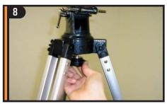
From underneath the tripod mounting platform, thread the attached mounting bolt into the hole on the bottom of the equatorial mount.
