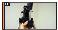
Thread the threaded end of the counterweight bar into the Dec axis of the equatorial mount.
