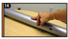
Before mounting the tube, remove the two wingnuts on the tube.
