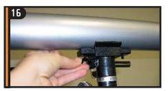
Reattach both wingnuts and tighten to secure in place. The front of the tube should be positioned over the counterweight assembly.
