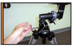
Thread the latitude adjustment screw into the equatorial mount until it is touching the inside of the mount.
