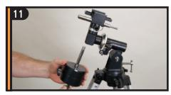
Thread the threaded end of the counterweight bar into the Dec axis of the equatorial mount.
