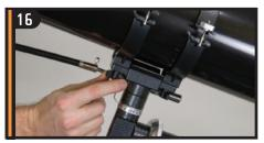
Reattach both knobs and tighten to secure in place. The focuser end of the telescope should be over the counterweight assembly.
