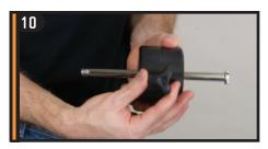
Locate the counterweight bar and counterweight. Slide the counterweight half way down the counterweight bar and tighten the locking screw to secure in place.
