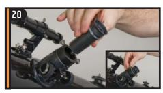
Insert the chrome barrel of the 20mm eyepiece into the focuser and tighten the screws.
