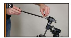
Slide the chrome end of the slow motion control cables onto equatorial mount gear shaft and tighten screw to secure in place.
