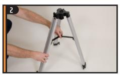
To set up the tripod, spread the legs outward until they are fully extended and push down center leg brace.
