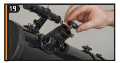
Loosen the screw on the focuser so that it does not obstruct the inner diameter of the focuser. Remove the plastic cap covering the end of the focuser.
