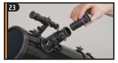
Place the eyepiece into the barlow and tighten the set screw to secure in place.
