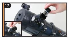
Insert the chrome barrel of the 20mm eyepiece into the focuser and tighten the set screw.
