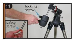
Remove safety screw from the end of the counterweight bar. Slide the counterweights half way up the bar and tighten the locking screw to secure in place. Replace safety screw.
