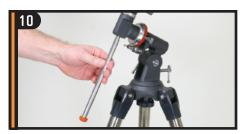
Tighten the threaded end of the counterweight bar into the Dec axis of the equatorial mount.
