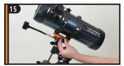
Center dovetail in the mount and tighten fastening screw. For added security tighten the angled lock down screw next to the fastening screw.
