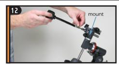
Slide the chrome end of the slow motion control cable onto declination axis gear shaft.
