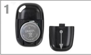
To insert or replace the battery, place your thumb in the center of the back cover, pressing inward and sliding downward remove the battery door. The CR2032 battery should be inserted with the positive (+) side facing upward. Replace the cover.
