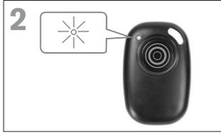
Press and hold the button on the remote for 5 seconds. A blue light will turn on and, after a few seconds, start to blink. The remote is now in pairing mode.
