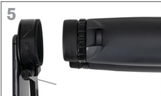
Fit the eyecup cuff over the eyecup of the binocular and tighten the eyecup cuff tension knob until the adapter is held firmly in place
