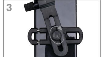
Tighten the smartphone clamp position knob and check that the position of the adapter's eyecup aperture stays centered over the smartphone camera lens
